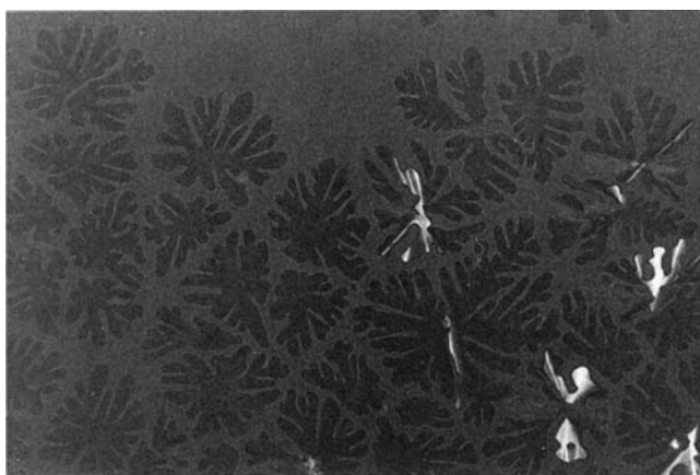
Figure 4. The dendritic formation of the D_{ho} mesophase of Pc 1 (220°C, 200× magnification, parallel polarizers).
