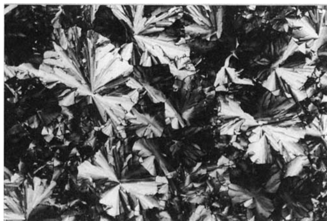
Figure 3. Optical texture of the D_{h0} mesophase of Pc 1 frozen into the solid glass state ( 18^\circ\text{C} , 200\times magnification, crossed polarizers).
